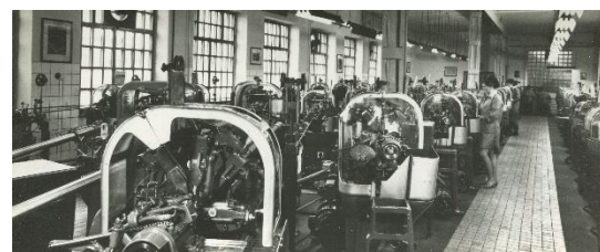
Fig. 4. Sliding head lathes in Nove mesto plant. Source: State municipal Archive Hradec Kralove
