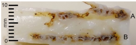
Fig. 8. Coagulated albumen phantoms, LEED = 80 J/cm (8 W, 1 mm/s) for 1470 nm (A) and 1940 nm (B).
