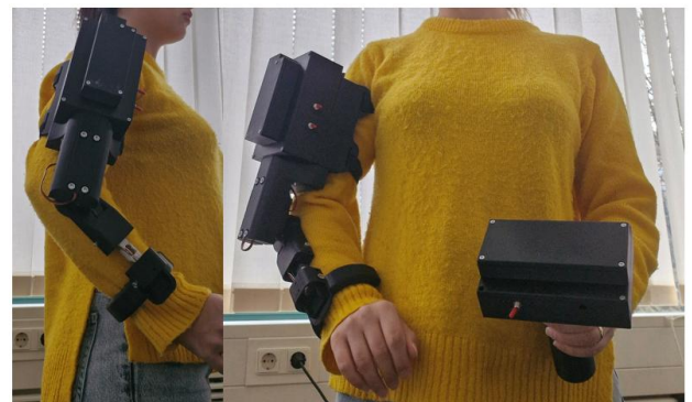
Fig. 6. Final prototype of the developed upper-limb exoskeleton worn by a user.
