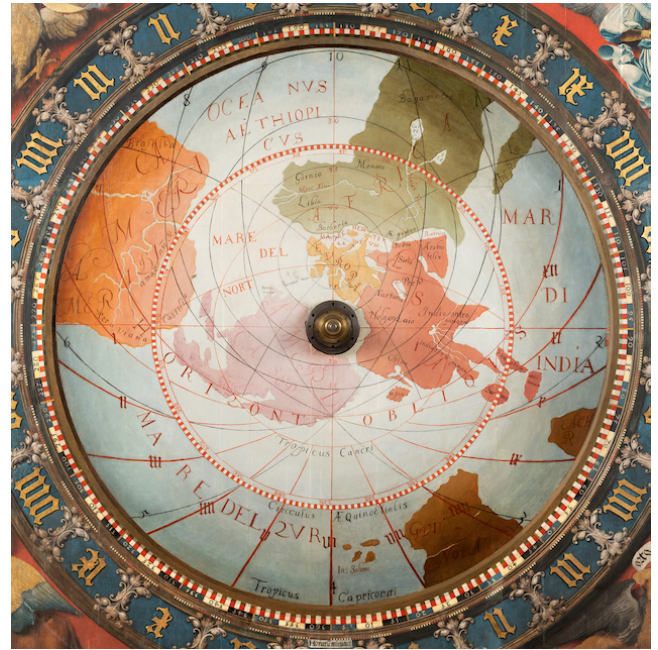
Fig. 3. Münster clock: geographic planisphere beneath the astrolabic rete, exposed during restoration after removal of the rete (©Stephan Kube, Greven)
